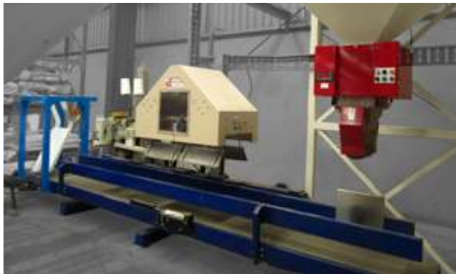
Bagging line filling woven poly and laminated woven poly bags with various free flowing products
