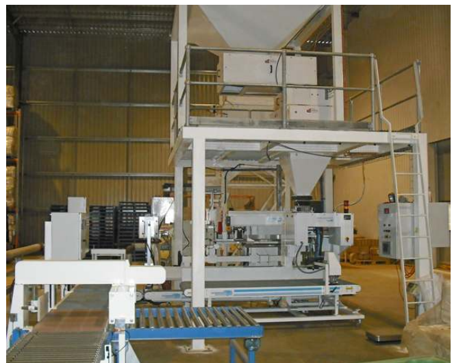
Belt fed Net Weighing over Total Bag Control system with T20 bag placer. Foreground showing check weighing and out of specification bag rejection system
