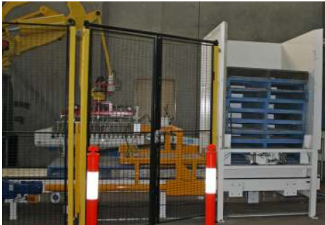
Automatic Pallet Feeder and Slip Sheet Applicator
