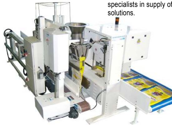
View of Total Bag Control Bag Filling and Sewing with bags presented for filling by T20MX SackPlacer
