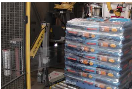
Automatic Stretch Wrapping of Filled Pallet
