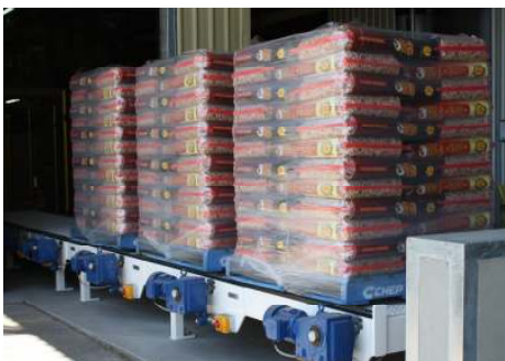
Filled and Wrapped Pallets on an Accumulation Line
