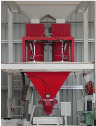
Duplex Net Weigher Bagging application
