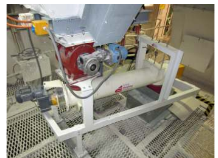
Pivoted Weigh Screw Feeder- Hydrated Lime application
