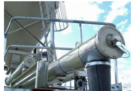
Pivoted Weigh Screw Conveyor- Cement application
