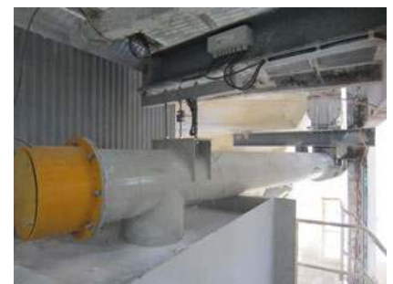
Pivoted Weigh Screw Conveyor- Malt Bulk Outloading application
