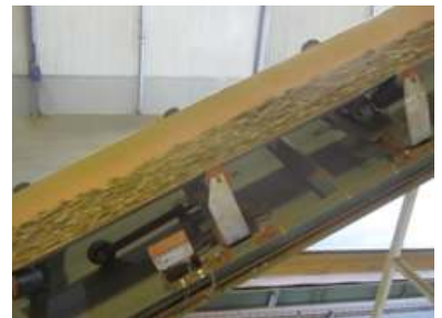
Twin Idler 600mm wide Belt Weigher - trough belt with 28 degree incline application
