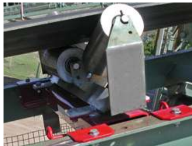
Single Idler 600mm wide Belt Weigher—trough belt application
