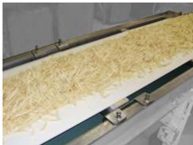
Single Idler 600mm wide Stainless Steel Belt Weigher application
