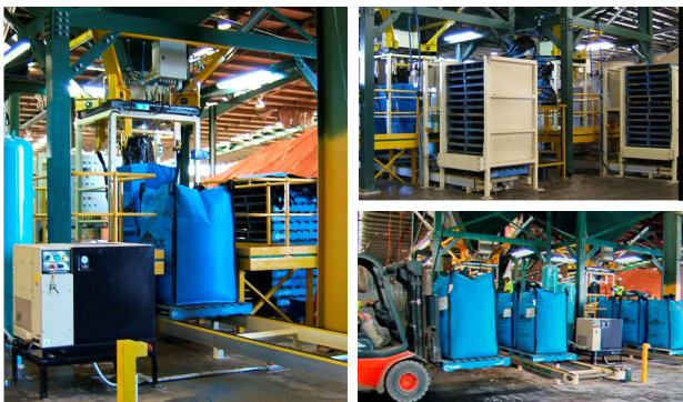
Dual 60tph Filling Lines with Automatic Pallet Dispensers and Accumulation Lines
